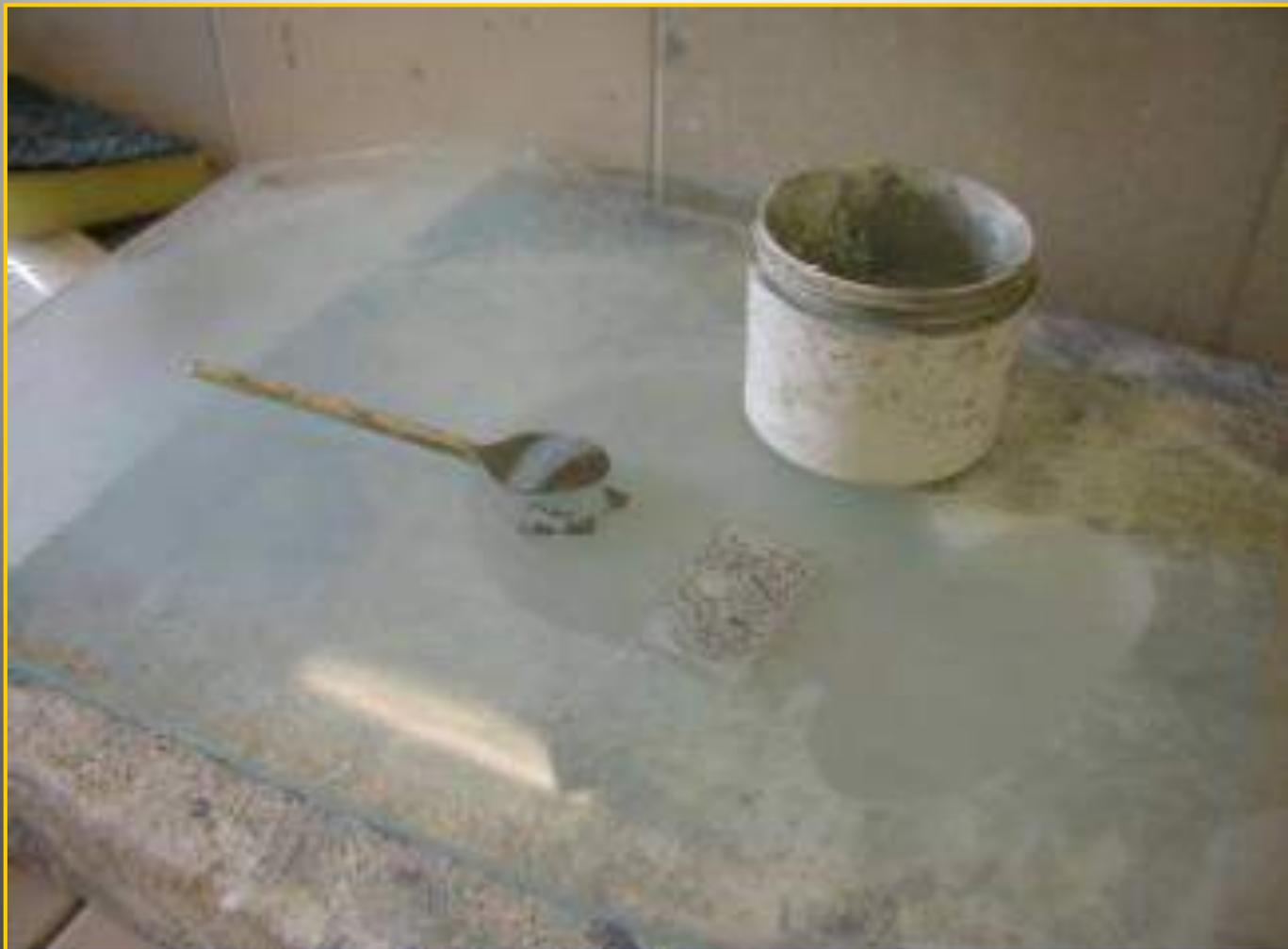
L'ULTIMO PASSAGGIO E' LA LUCIDATURA FINALE EFFETTUATA SIA A MANO (CON PASTE ABRASIVE SU UNA LASTRA DI VETRO).....
